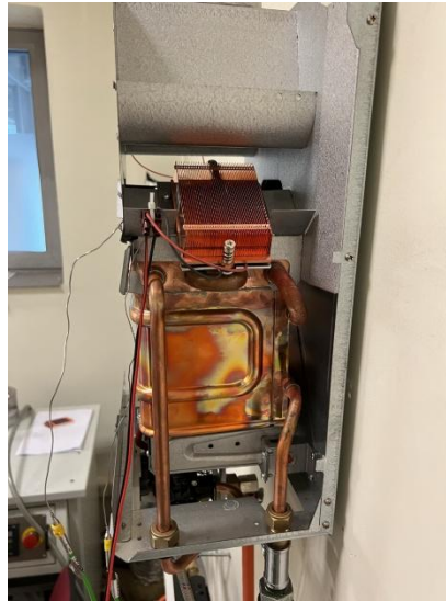
MicroTEG for powering the control system of a domestic heater
