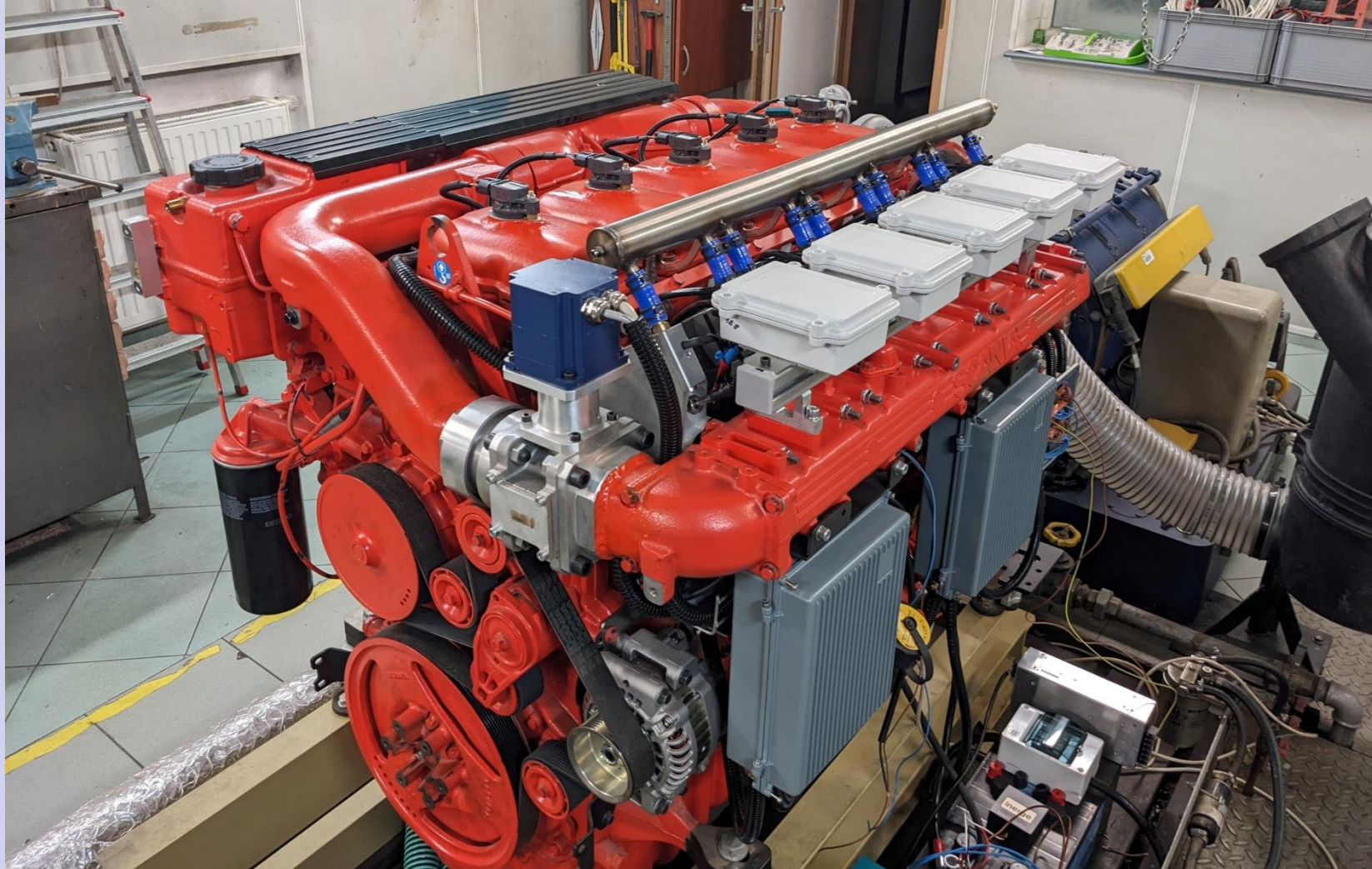
Scania engine during tests at the laboratory of the Cracow University of Technology
