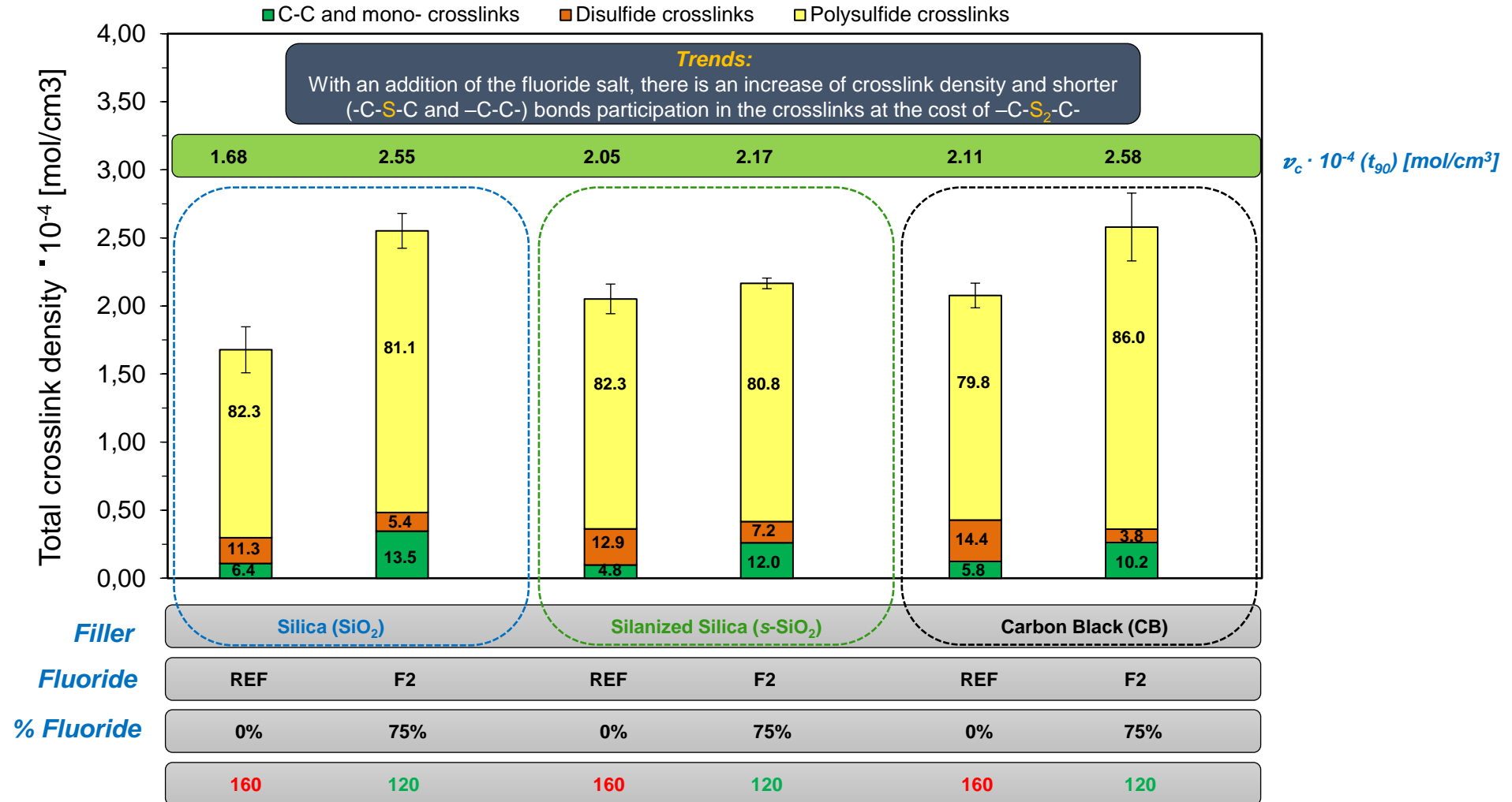
Crosslink density and structure – filled NBR compounds; comparison of fillers
